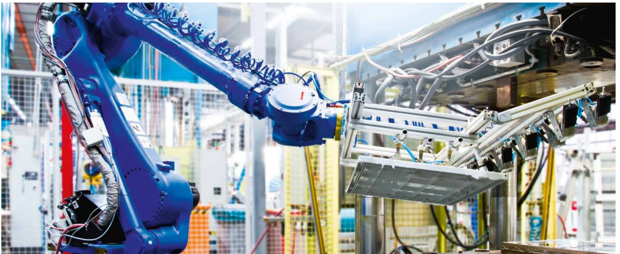
Mitras specifically developed an automated solution for the PIMC process for series production.
